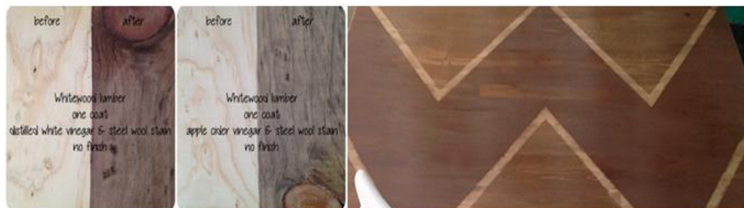
Fig (8) Distilled white vinegar gave the wood sample a reddish/brownish hueWhilst the apple cider vinegar stained the wood a grayish color.
